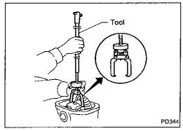
4. Lift differential case assembly out with Tool. Tool number: HT72400000 ( — )
