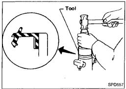
Apply multi-purpose grease to cavity at sealing lips of oil seal. Install front oil seal with Tool.
