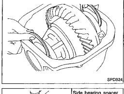
12. Drive in side bearing spacer with Tool. Tool number: KV38100600 (J25267)
