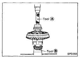
Press-fit side bearing inner cones on differential case with Tool.
