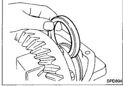
3. Put the side bearing spacer in place on the ring gear end of the carrier.
