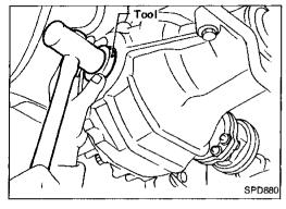
Apply multi-purpose grease to sealing lips of oil seal.
