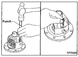
Install pinion mate shaft lock pin with a punch. —R200 ONLY—
