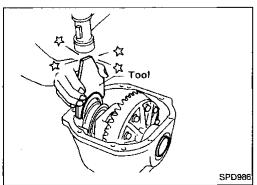
Using Tool side bearing spacer drift, place both of the original carrier side bearing preload shims on the carrier end, opposite the ring gear.
