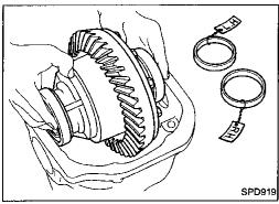
Keep the side bearing outer races together with inner cone — do not mix them up.
