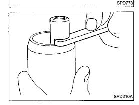
Select the correct thickness of pinion bearing preload adjusting washer using a standard gauge of 3.5 mm (0.138 in) and your J34309-101 feeler gauge. The exact measure you get with your gauges is the thickness of the adjusting washer required. Select the correct washer from the following chart.
