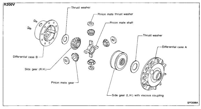
For quiet and reliable final drive operation, the following five adjustments must be made correctly.
