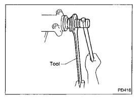
Install companion flange, and tighten pinion nut to specified torque with Tool.
