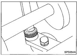
12. Select the correct standard pinion height adjusting washer thickness using a standard gauge of 3 mm (0.12 in) and your J34309-101 feeler gauge. Measure the distance between the J34309-11 pinion height adapter including the standard gauge and the arbor.
