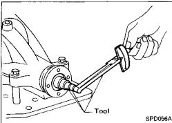
Turn drive pinion in both directions several times, and measure pinion bearing preload.
