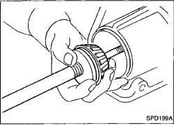
4. Assemble the front pinion bearing inner cone and the J34309-2 gauge anvil together with the J34309-1 gauge screw in the final drive housing. Make sure that the pinion height gauge plate, J34309-16, will turn a full 360 degrees, and tighten the two sections together by hand.
