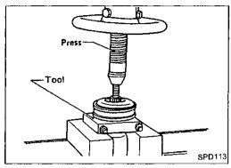
5. Remove center bearing with Tool and press.
