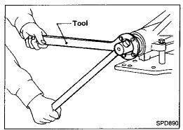
5. Loosen drive pinion nut and pull off companion flange.
