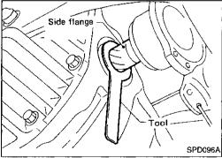
5. Install final drive side flange with Tool.
