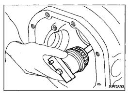
3. Place the pinion preload shim selector Tool, J34309-1, gauge screw assembly with the pinion rear bearing inner cone installed into the final drive housing.
